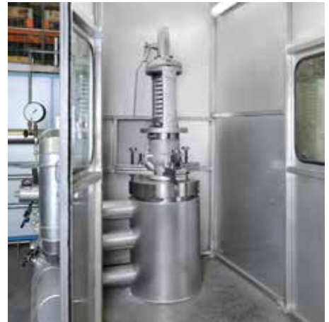
IMI Bopp & Reuther operates 2 steam test benches for hot setting of steam safety valves
