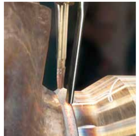
Seal welds with the highest accuracy between nozzle and body
