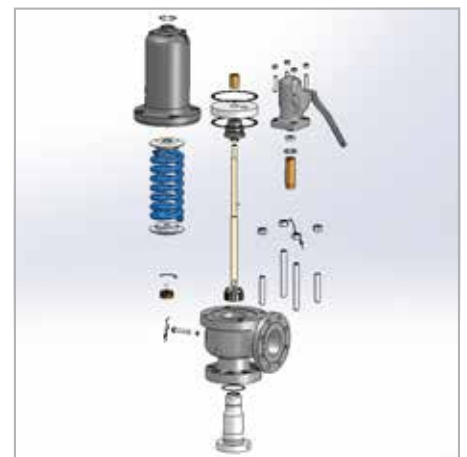
Explosion view of API valve shows inner and outer parts.
