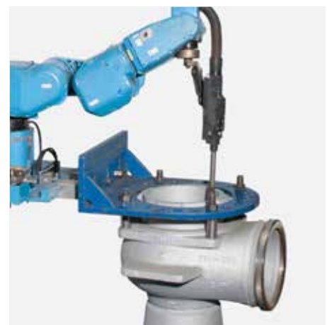
IMI Bopp & Reuther does possess the technology to perform high quality body seat repair.
