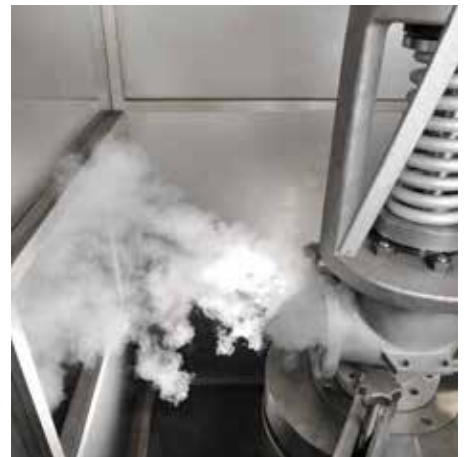
IMI Bopp & Reuther operates 2 steam test benches for hot setting of steam safety valves
